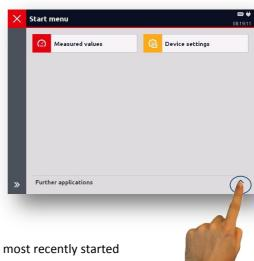
Using the button in the "Further applications" field, additional functions or applications of the device will be shown for selection:
