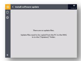
Update files for the device always have to be transferred manually from the PC to Updates". Multiple update files can be saved to the device at the same time.
