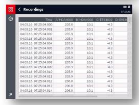
In the Recording menu you can switch between the graphical view and table view at any time, also with event logs.
